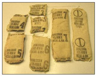
**Figure 5, 105mm Propellant Increments**
