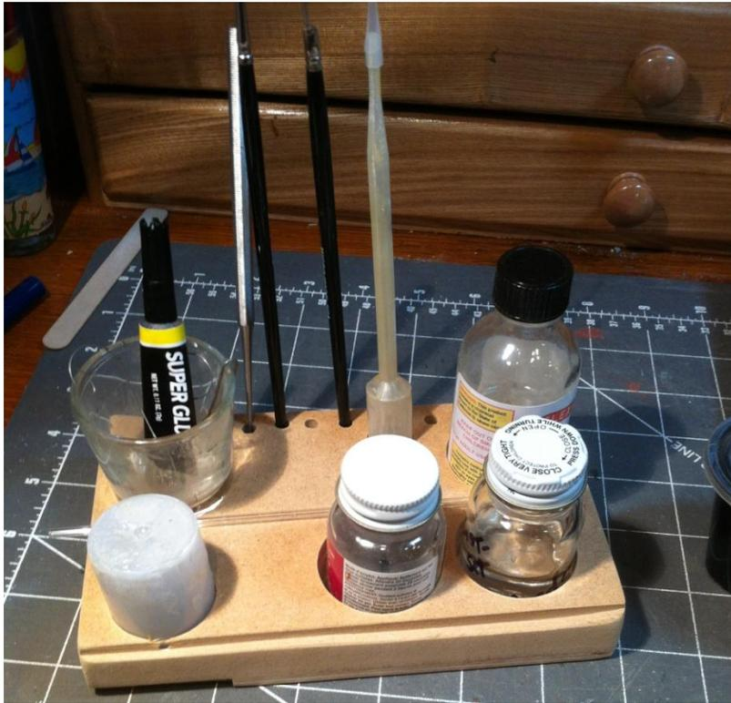
From left, back row-- super glue holder (an old jigger), accelerator applicator, superglue applicator, eye dropper for liquid glue, touch-n-flow glue. Front row, old 35mm film case for superglue, Testor's liquid glue, super glue accelerator (in old Testor's container). In the middle is the touch-n-flow applicator.
