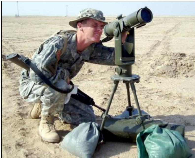
**Figure 12, Emplaced Collimator**
